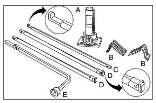
The tools you'll be using include the bottle jack (A), the wheel blocks (B), the jack handle (C), the jack handle extensions (D), and the wheel wrench (E).
